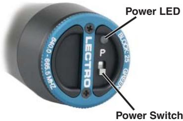
**IMPORTANT:** When performing the following steps, The transmitter allows ten seconds to set the frequency switches before the next toggle of the power switch. When toggling the power switch, it is not necessary to allow the transmitter to turn off completely. If more than ten seconds elapse between toggles, the mode change will not take effect and you must begin again from step 3.
