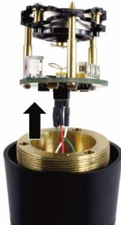
6) Set new capsule assembly to align the holes for the socket head bolts
