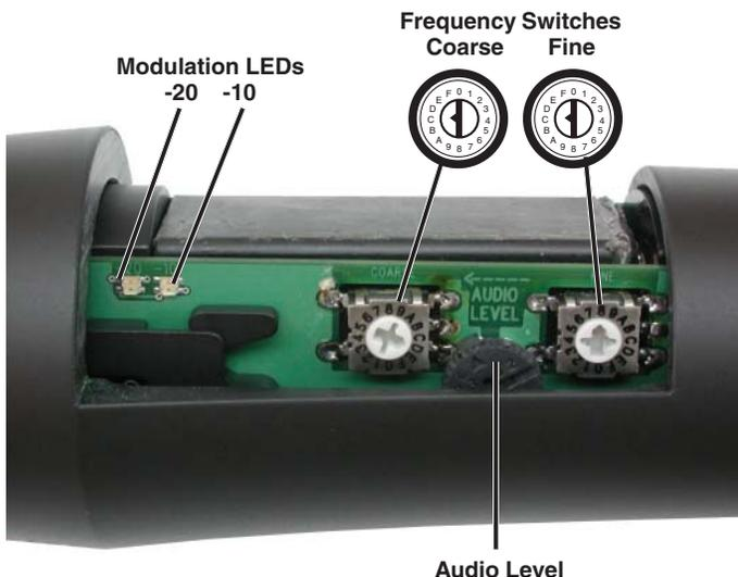
4) Rapidly toggle the Power Switch Off and On. Change the Frequency Switches to one of the following settings:
